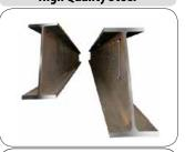
Constructed with 100,000 psi yield strength steel for the side rails and main beams. The high tensile steel ensures the designed camber is retained, and allows for a longer product service life.
